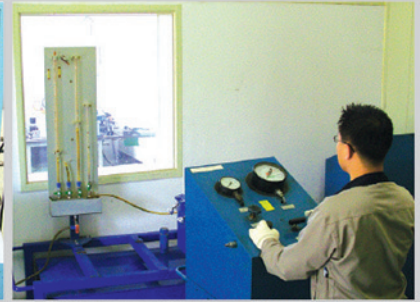
검증압(3000PSI)시험 Certified Pressure(3000PSI) Test
