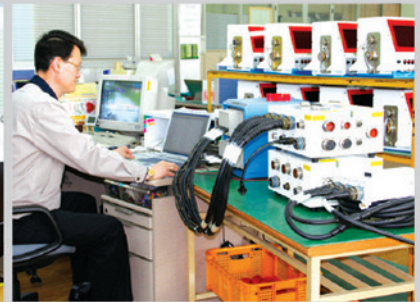
배선절연검사 Wiring Insulation Test
